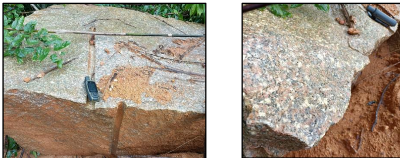
Figure 4: Semi-drill holes in RT from granite block cutting
