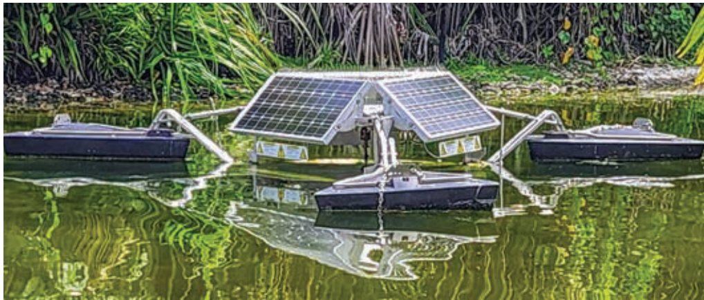
Figure 8: SolarBee water purifier at Pullman Maamutaa Resort natural lake.
