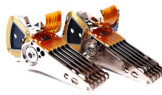
Actuator Pivot-bearing Flex-circuit Assembly
