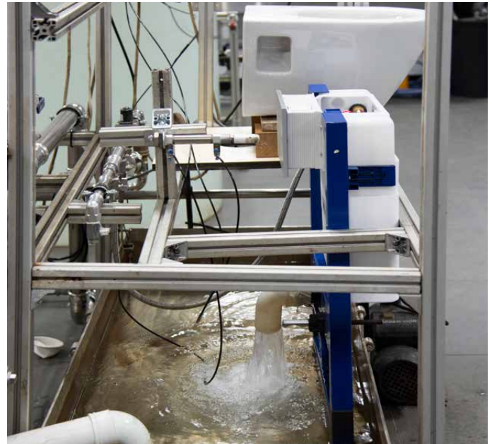
Recycling of water for sanitary ware testing under Water Efficiency Labelling Scheme (WELS).
