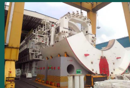
TBM shield under construction
