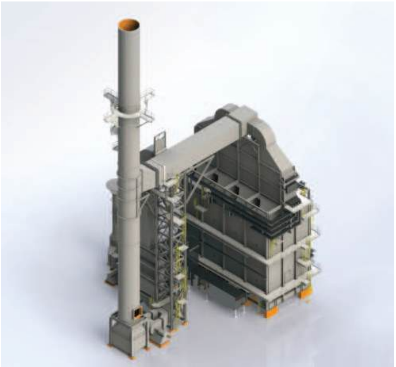
3D visual of a hydrogen-fired crude oil heater for an O&G client
