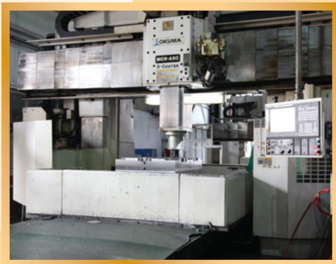
加工中心正為一件大型模架進行加工 A CNC machining centre is processing the machining process for a large size mould base
