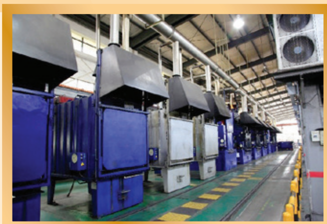
多用途熱處理爐可提供各種不同的熱處理加工服務 Multi-purpose heat treatment furnaces can provide various kinds of heat treatment services
