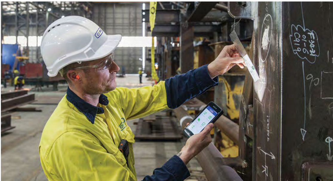
Civmec's Civtrac barcode tracking system
