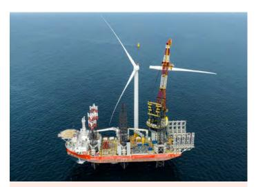
Cadeler's offshore wind turbine installation vessel
