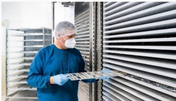
Figure 3 Loading freeze dryer
