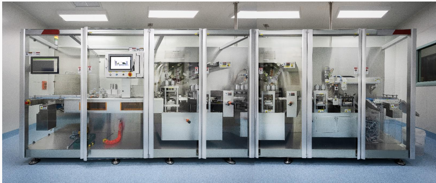
Figure 2 Automated sealing, packaging and inspection line
