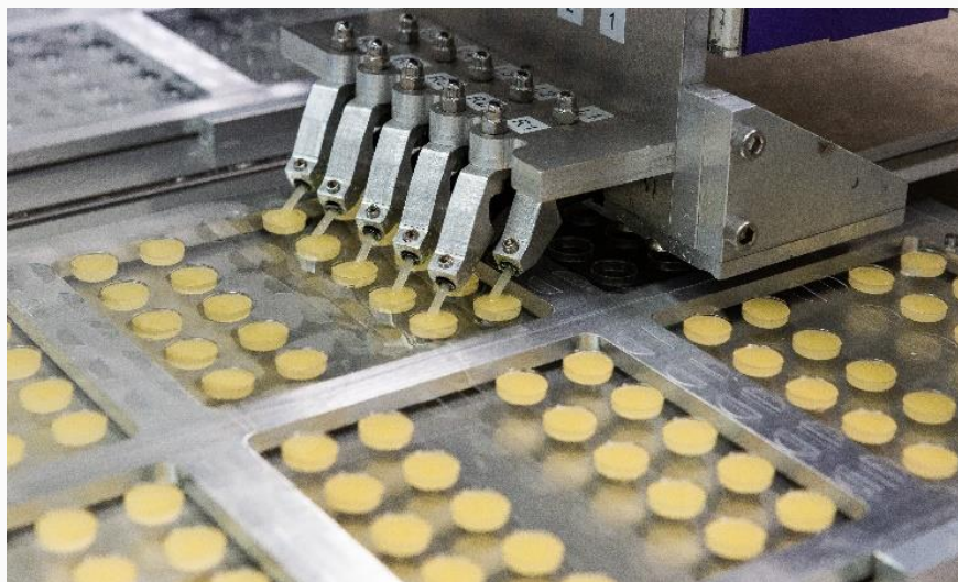
Figure 6 Blister filling for wafer production
