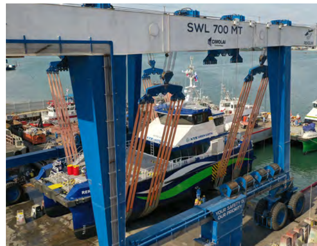
A WindFlex-27 CTV being launched at PT Kim Seah with a 700 MT marine travel lift.
