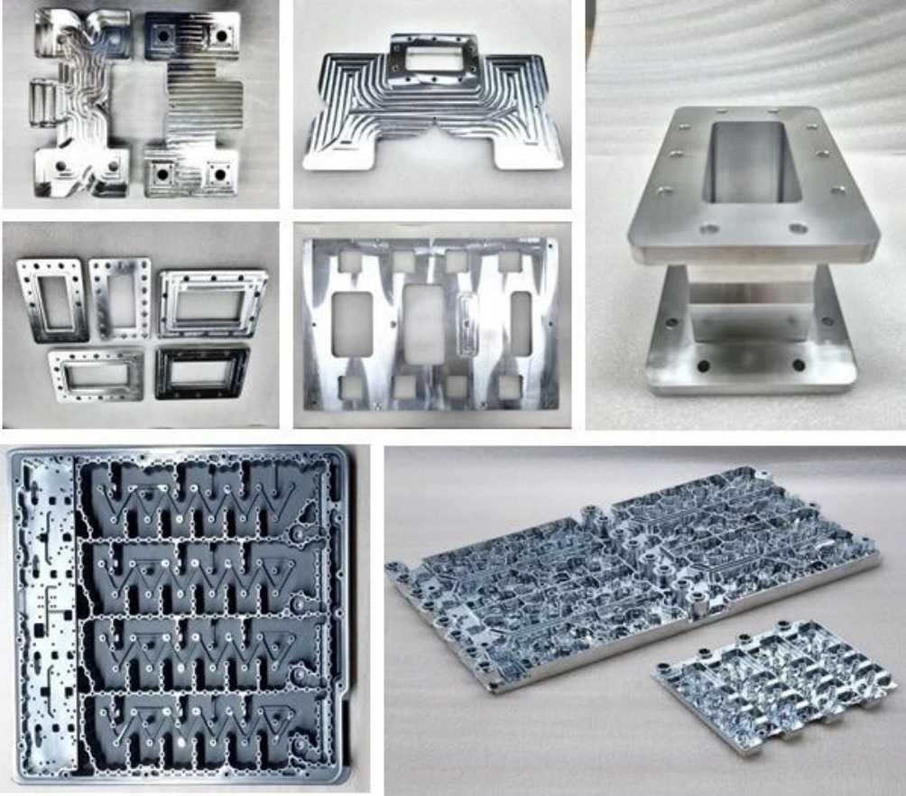
Machined parts for wireless infrastructure and microwave energy product
