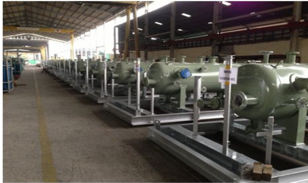
WHS SHIPMENT 23, 12 Vessels Mounted on Skids, Pipe Fit Ups Commenced
