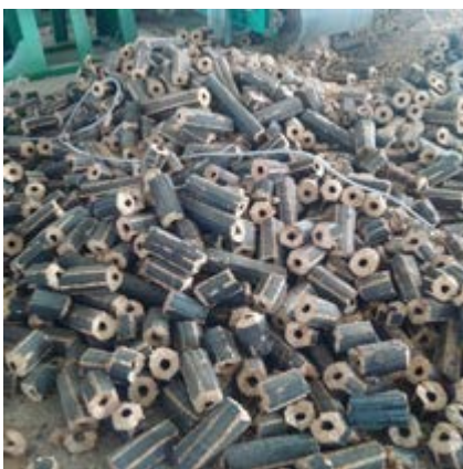
Production of briquettes during plant commissioning
