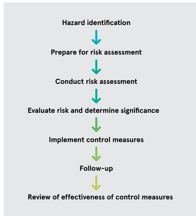
Diagram 1. Procedure outline of hazard identification and risk assessment conducted thrice a year
