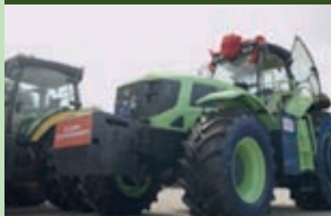
GYMCL 350-horsepower hybrid electric CVT powertrain in Liugong Tractors
