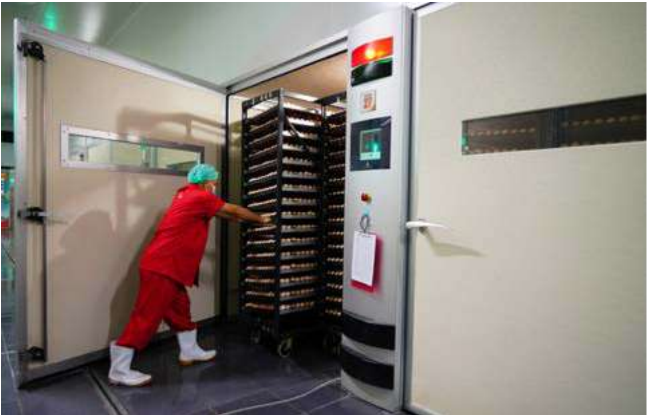
Mesin Setter di Unit Penetasan Telur Setter Machine in Poultry Hatchery Unit
