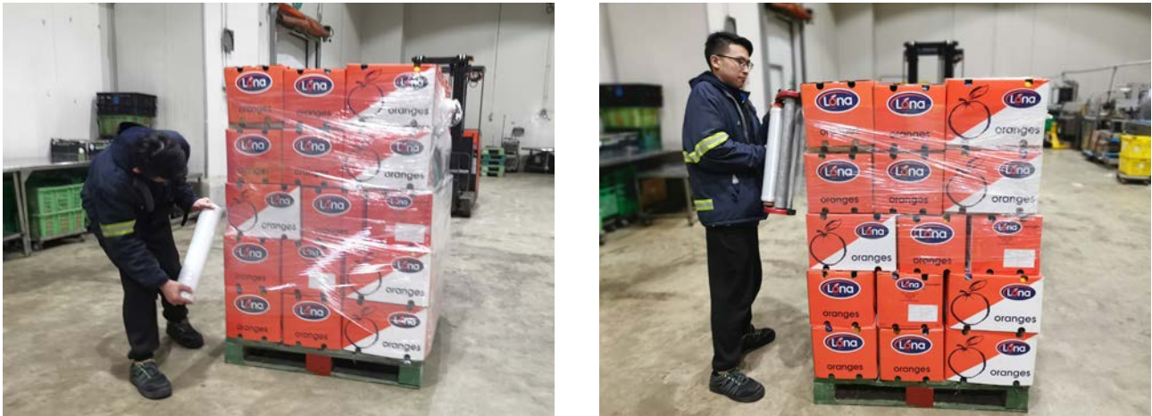
Our adoption of a newer assisted pallet wrapping system with a handheld tool (right) has enabled us to optimise our stretch film use and reduce our staff's workload.
