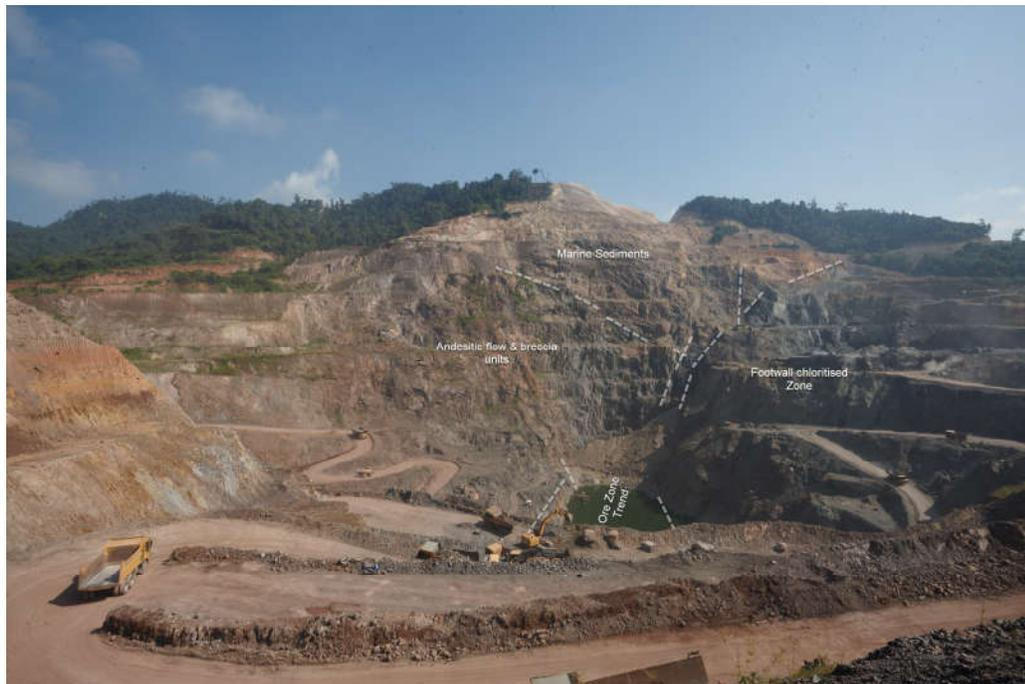
**Figure 3,** View looking NW, capping marine sediments over hosting andesitic volcanics
