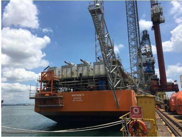
Stern of Ingenium II with flare stack, crude offloading station and power gen sets
