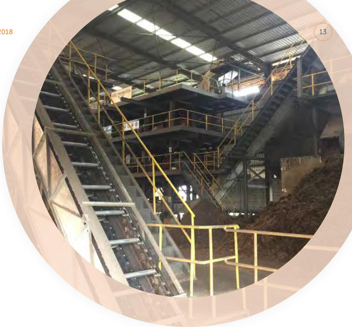
“ In Mewah Datu Sdn Bhd, we utilize the fiber from empty fruit bunch (EFB) and palm kernel shell (PKS) as boiler fuel to replace fossil fuel. The EFB and PKS are the solid waste from oil palm obtained from milling process. This agricultural waste is considered to have zero life-cycle greenhouse gas emissions up to the point of collection.
