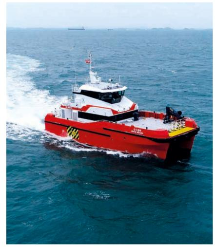
sufficient confidence to start a **Built to order:** 26m Crew Transfer Vessel for offshore wind.
