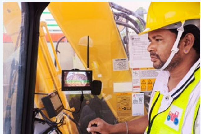
Using an artificial intelligence sensor in excavators for greater safety.
