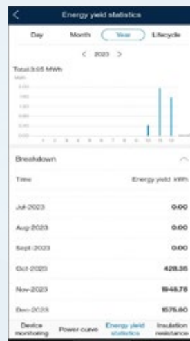
Data extracted from the solar photovoltaic monitoring system
