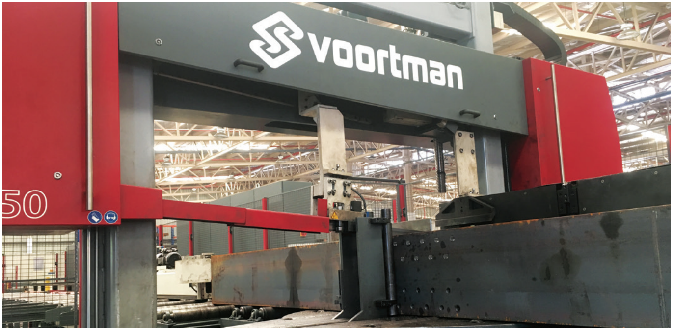
Fully-automated steel structure fabrication processing line at the Tuas Manufacturing Hub in Singapore.
