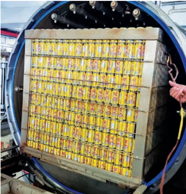
Yeo's China Guangzhou Plant adopts Retort Low Energy Suction System (L.E.S.S.) to lower water consumption
