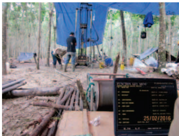
Figure 4:4 WRL Down-hole Geophysical Logging Operations
