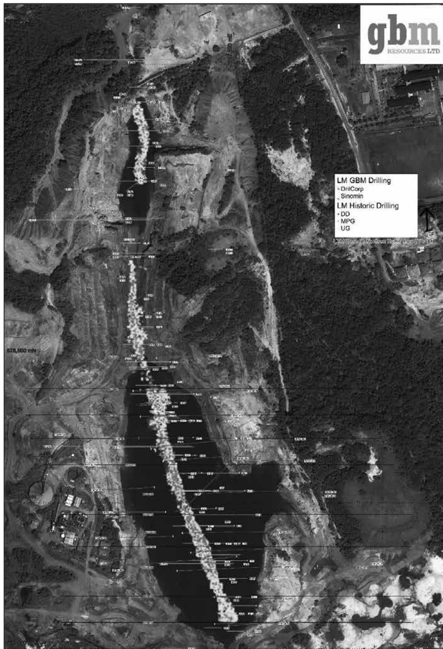
Figure 6.1 Lubuk Mandi Mine drillhole locations relative to gold mineralisation
