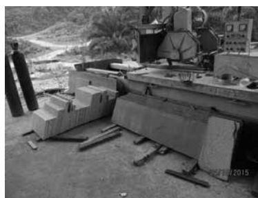
Figure 1-1; Previous extraction of dimension stone at Bukit Chetai with production of floor and wall tiles
