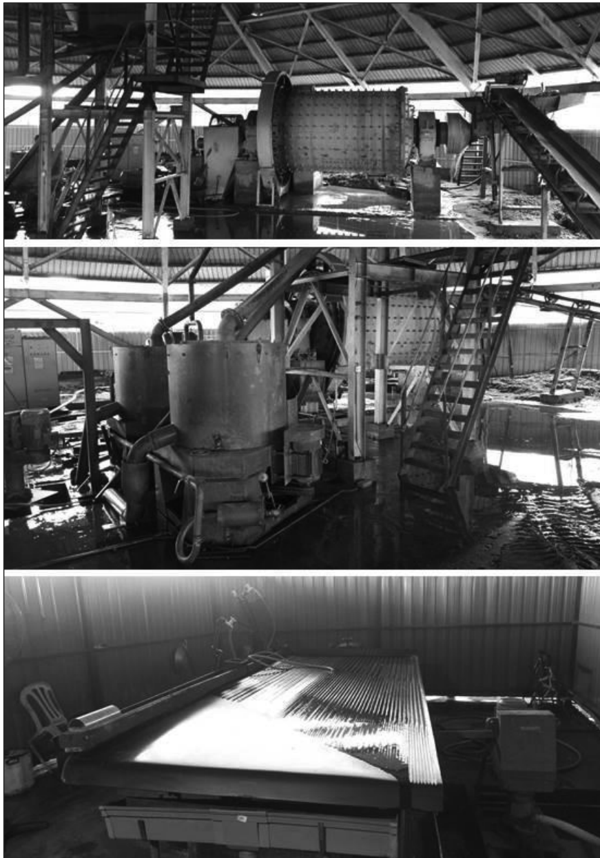
Figure 11.3: Ball mill (top), Knelson concentrators (middle), shaking table (bottom)
