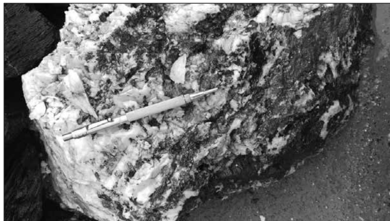
Figure 5.4 Mineralised quartz vein material at the Lubuk Mandi Mine
