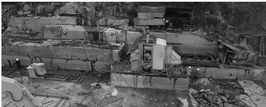
Figure 5-2; New quarry faces developed for utilization of circular saw
