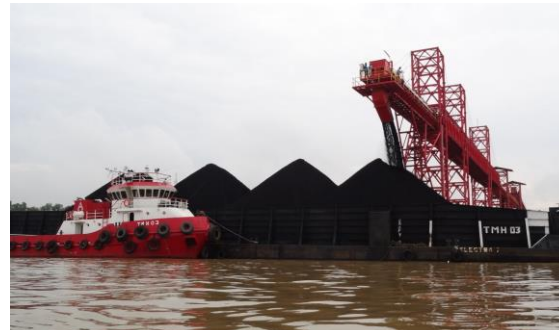
Coal Being loaded onto Barge via Conveyor at Jetty
