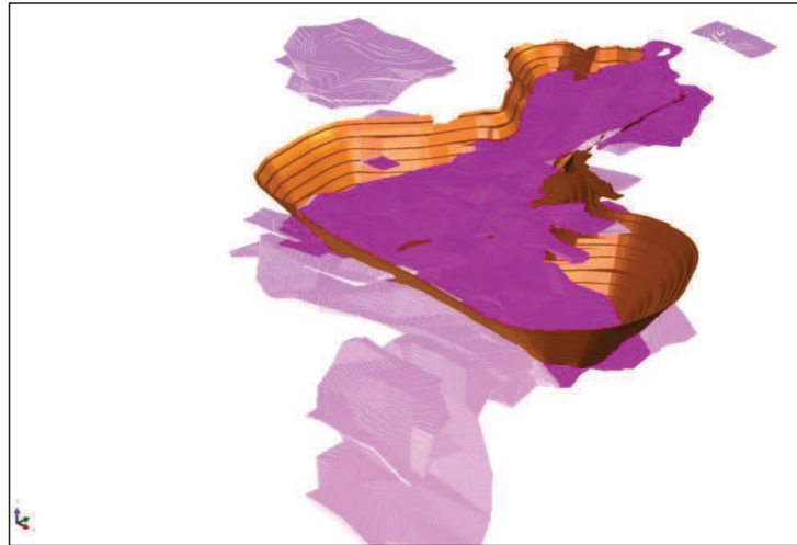
Figure 38: Oblique view of latest pit design (dark magenta = Indicated, light magenta = Inferred, mineral resources)
