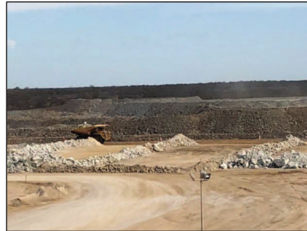
Run of Mine stockpile fingers
