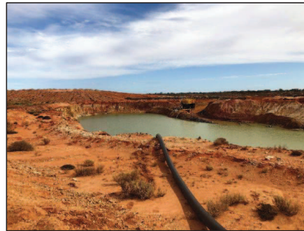
Water re-circulation via historical pits and lines
