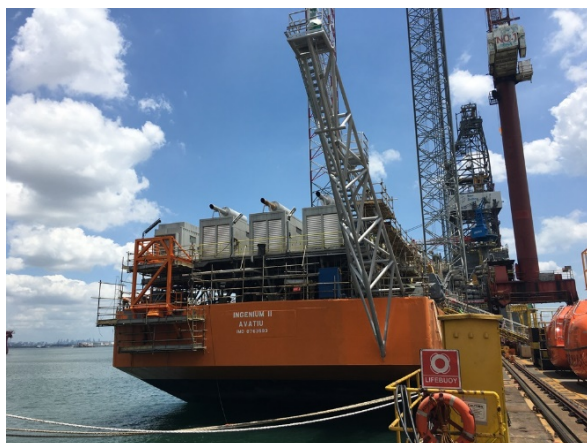
Stern of the Ingenium II production barge showing flare stack, crude offloading station and power gen sets
