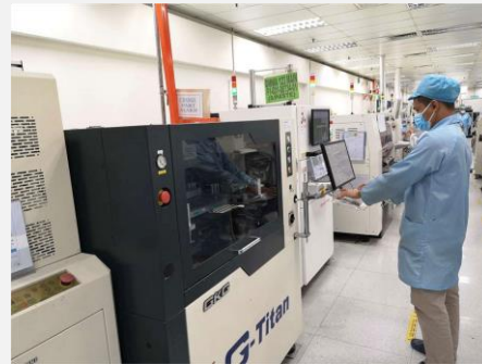
Figure 4: Demonstration of 3D AOI high-tech machinery by SMT department
