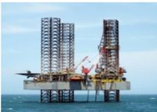
**JACK-UP RIG** is a mobile self-elevating drilling platform equipped with legs that can be lowered down to the ocean floor.
