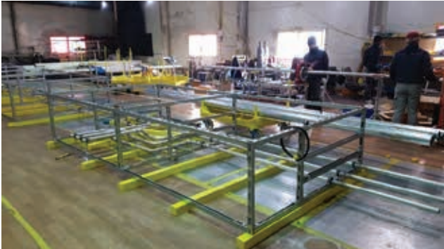
DfMA – Pre-connection between Mechanical, electrical and plumbing service modules
