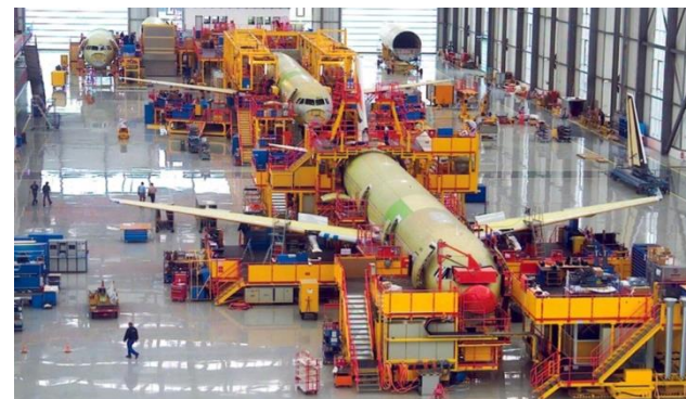
A320 Family Final Assembly Line in Hamburg
