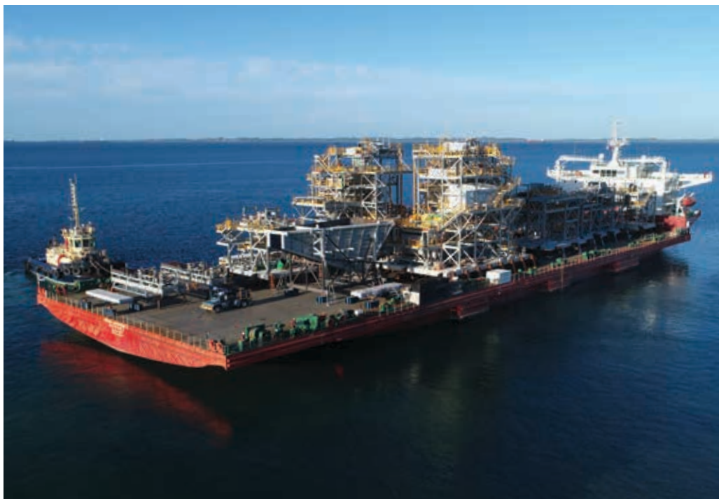
Beneficiation modules being shipped to Amrun project in Queensland
