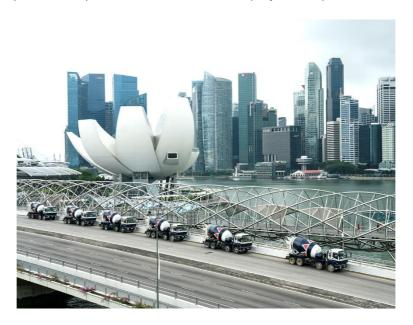
Pan-United's AiM in-transit concrete management system calibrates the consistency of concrete in mixer trucks. This increases product quality consistency among mixer trucks and minimises the number of workers and employees required on-site to test and approve the concrete quality.
