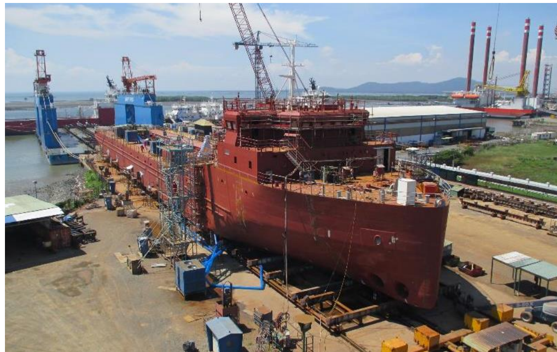
MCV for Topaz Energy and Marine under construction at Vard Vung Tau
