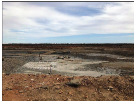
Blast hole drilling
