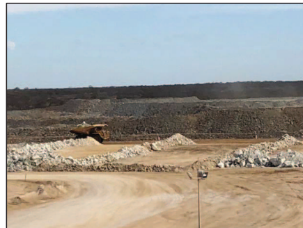
Run of Mine stockpile fingers
