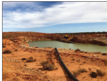
Water re-circulation via historical pits and lines
