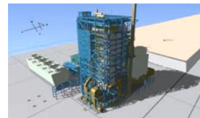
Conceptual drawing of the biomass boiler that makes use of pulp waste byproduct from the pulping process
