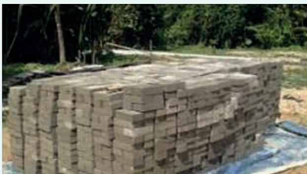
Hand made bricks constructed using crushed glass, clay and sand
