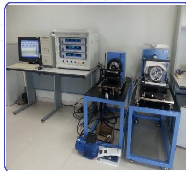
Loading Machines And Analyzer
