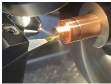
Five-axis diamond lathe <100 nm Contour accuracy
