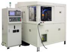
Five-axis diamond lathe <100 nm Contour accuracy
