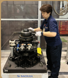
▶ An SIAEC senior technician securing a 787 Electrical Brake onto the test fixture to prepare for functional tests
