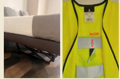
Bed lift used in property (left) and vest fitted with buzzers to alert user to maintain safer postures (right)
