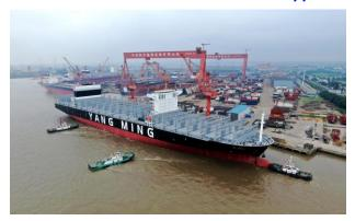
Measuring 332 meters long and 48 meters wide, the 12,600TEU containership was designed and built with world-leading specifications in terms of reliability and efficiency.
