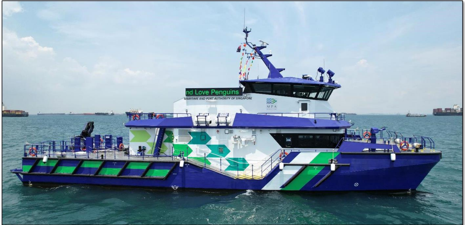
35m Hybrid-Electric Patrol Boat Delivered 1 unit to the Maritime and Port Authority of Singapore
