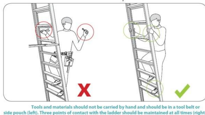
Figure 9. An illustration on using ladders safely in Asiatic's Fall Prevention Plan
