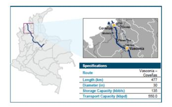
Segment III currently has an installed transport capacity of 550 kbpd. In accordance with the methodology established by the MME, the current tariff for Segment III is US\$3.3947/bbl.
