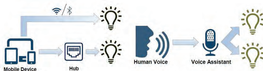
Figure 4-2: Control and Functionality of Smart LED bulbs
