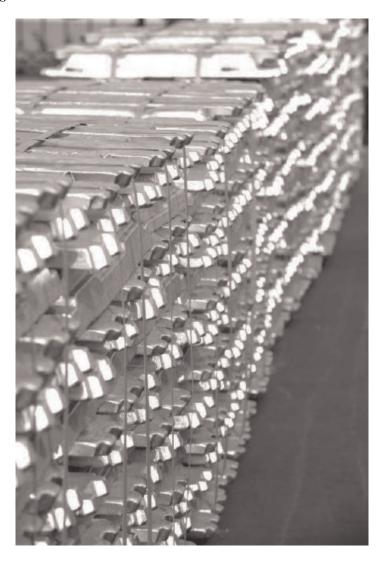
Sales of aluminum alloy ingots accounted for approximately 12.0%, 4.5%, 5.8% and 2.8% of our revenue for 2017, 2018 and the six months ended June 30, 2018 and 2019, respectively. Molten aluminum alloy is processed into aluminum alloy ingots through molding, casting and cooling. Our aluminum alloy ingots are produced by using self-manufactured molten aluminum alloy.
